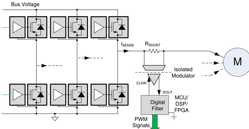
**Figure 4. Current Measurement Using an Isolated Modulator**
