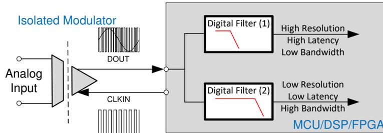
**Figure 3. Implementation of Two Digital Filter in Parallel**
