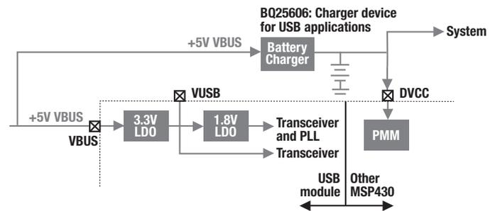
**Figure 4.** Power over USB can also be used as a primary source to charge batteries. TI's BQ2560x and BQ2407x charger families have been specifically designed for USB battery charging applications.
