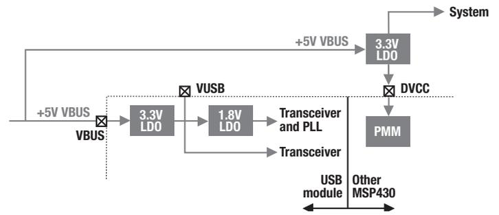
**Figure 3.** For high-current systems or for applications where it makes sense to power a device from battery even when connected via USB, the MSP430 offers the flexibility of bypassing the integrated 3.3V LDO and driving DVcc from an external supply.
