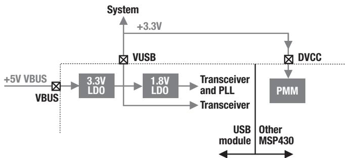
**Figure 2.** MSP430 USB microcontrollers can source power off the USB bus to power the entire system with 12 mA.
