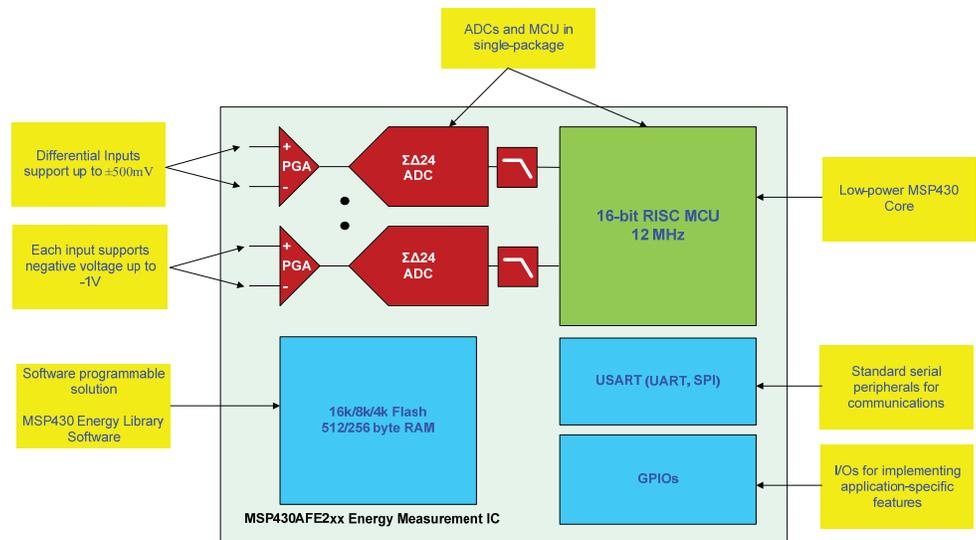
Figure 5: Features of the MSP430AFE2xx for energy-measurement applications
