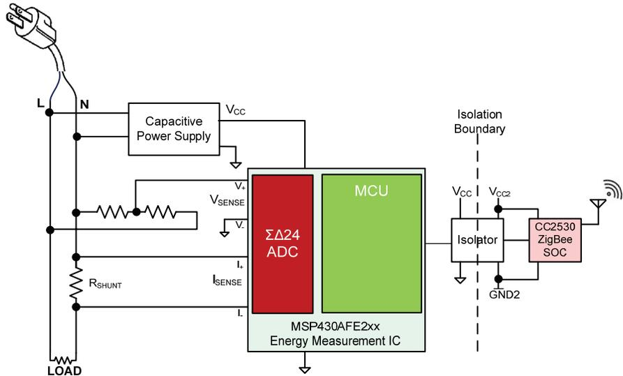
Figure 2: Block diagram of an energy measurement system
