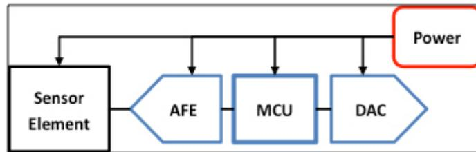
Figure 2: Block diagram of a current loop transmitter
