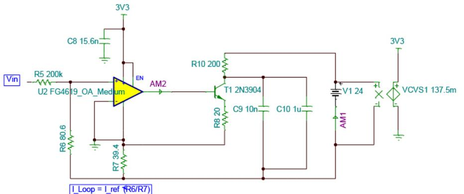
Figure 1. Schematic of a voltage-controlled current source
