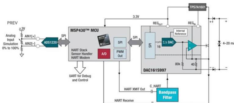
Figure 3: **Field transmitter featuring HART® communications**
