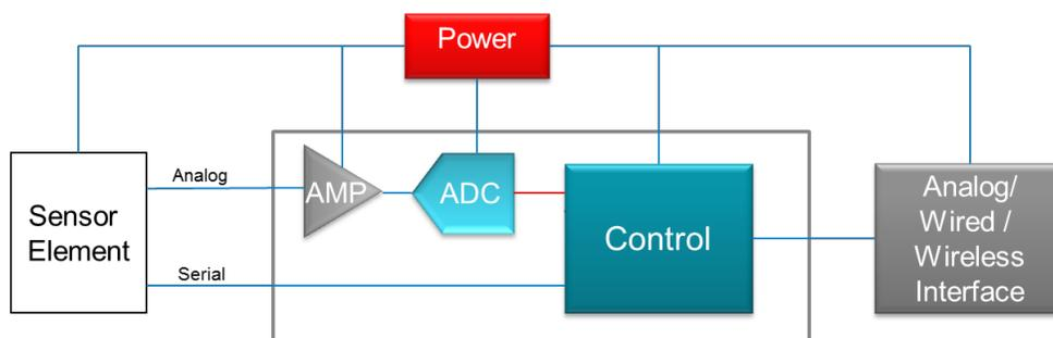
Figure 1: A typical industrial sensing system
