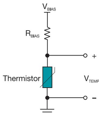
**Figure 2.** Thermistor placed in a voltage divider configuration.
