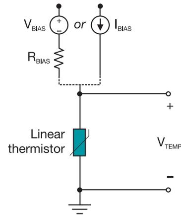
**Figure 6.** A linear PTC thermistor eliminates the need for a parallel resistor.
