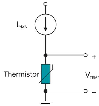
**Figure 3.** Thermistor biased with a constant current source.
