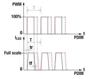
Figure 9. LED illumination with PWM dimming.
