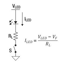
Figure 3. An LED driving circuit with a current-limiting resistor.
