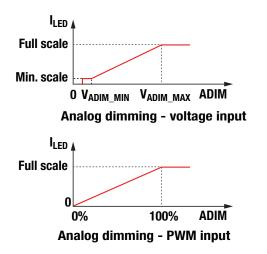
Figure 8. LED illumination with analog dimming.
