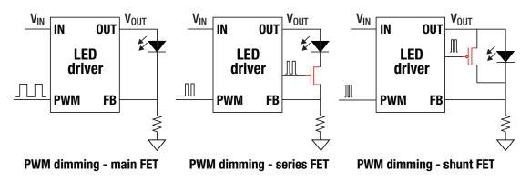
Figure 10. LED illumination PWM dimming methods.
