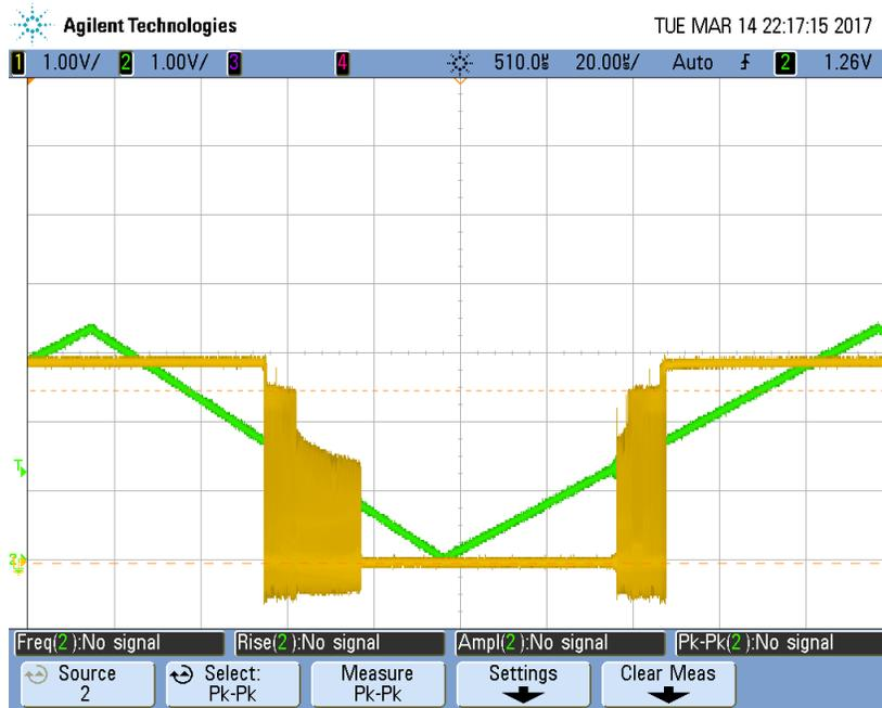
Figure 12. Waveforms Without Schmitt Trigger- SN74LVC1G34
