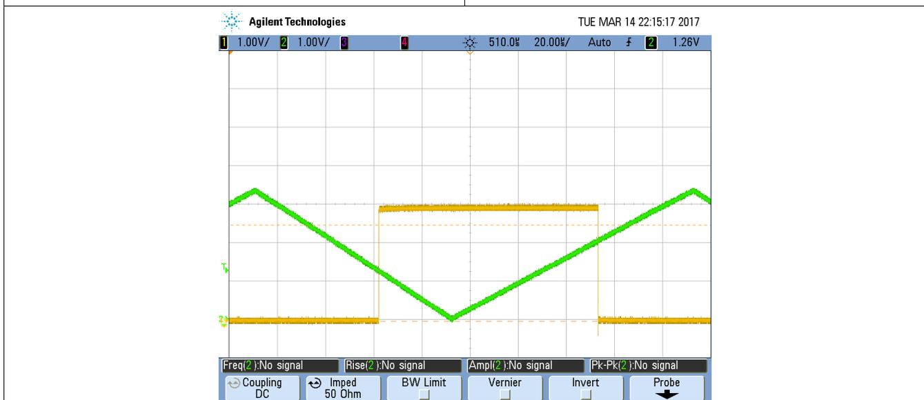
**Figure 16. Lab Setup Comparison With Schmitt Trigger SN74LVC1G14**
