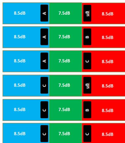
Figure 6. USB 3.1 Gen 2 10Gbit/s Insertion Loss Budgets
