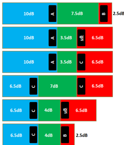
Figure 5. USB 3.1 Gen 1 5Gbit/s Insertion Loss Budget
