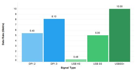
Figure 1. USB-C Signals and Their Associated Data Rates
