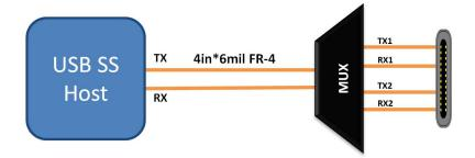
Figure 10. Illustration of a Small System Such as a Smartphone
