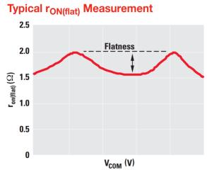
Figure 2. Device R<sub>on</sub> vs. Signal Voltage
