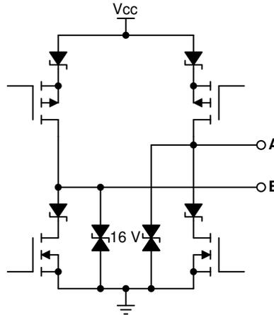
Figure 2-1. Differential Output Driver Structure
