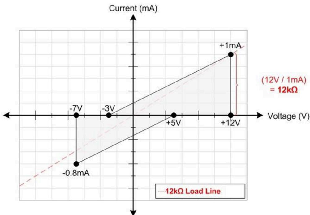
Figure 4-3. RS-485 Receiver Input I-V Characteristic
