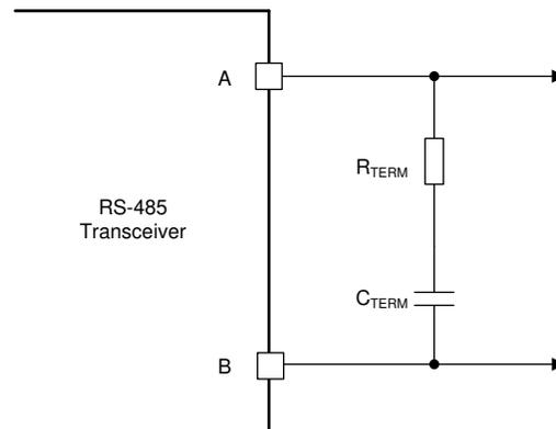
**Figure 6-3. AC Termination Network**
