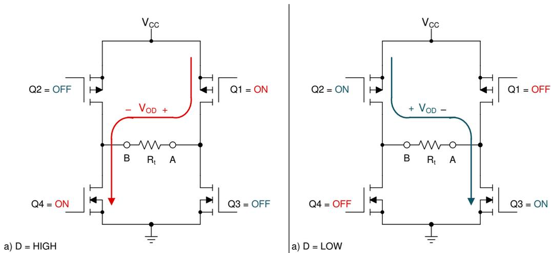
Figure 2-2. RS-485 Output Driver Operation
