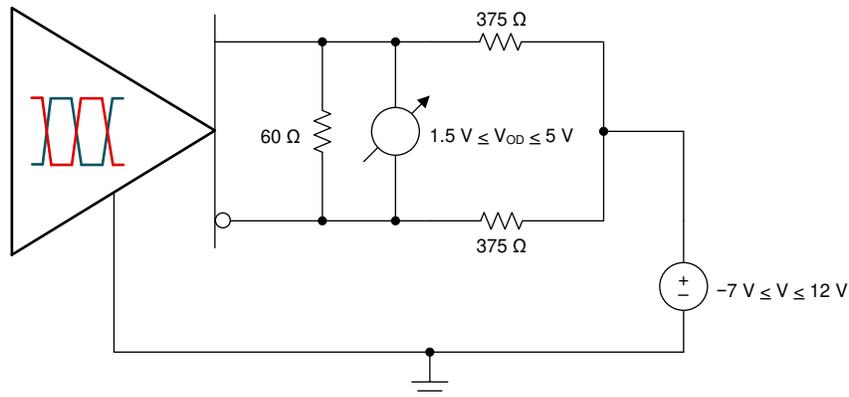
Figure 2-5. RS-485 Output Driver Test Circuit Over Common-Mode
