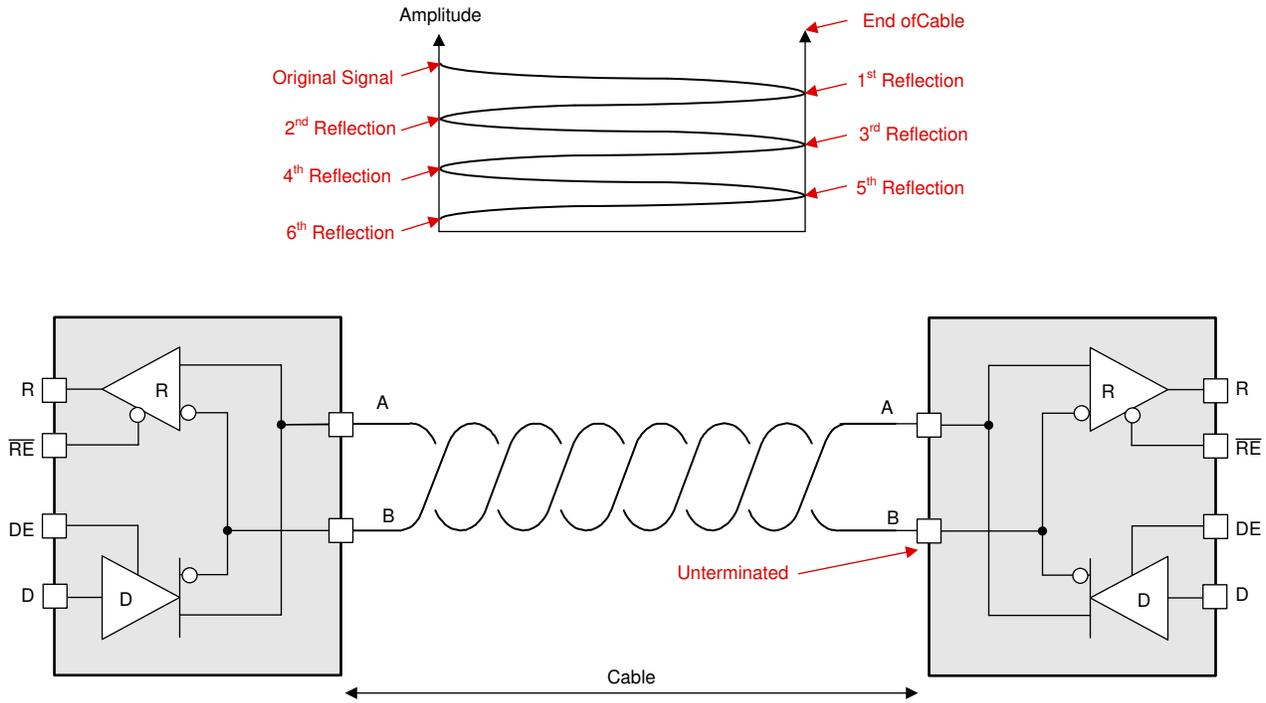
**Figure 6-1. Amplitude of Reflection Decay Each Time a Reflection Occurs**
