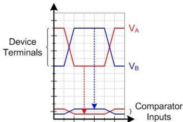
Figure 4-2. Receiver Input-Voltage Attenuation
