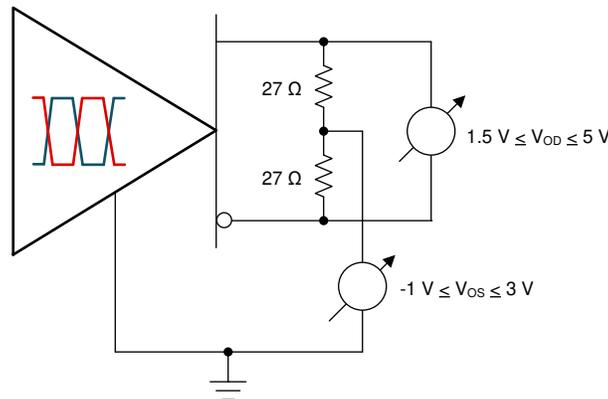
Figure 2-4. RS-485 Output Driver Test Circuit
