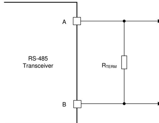
**Figure 6-2. Standard Termination Network**
