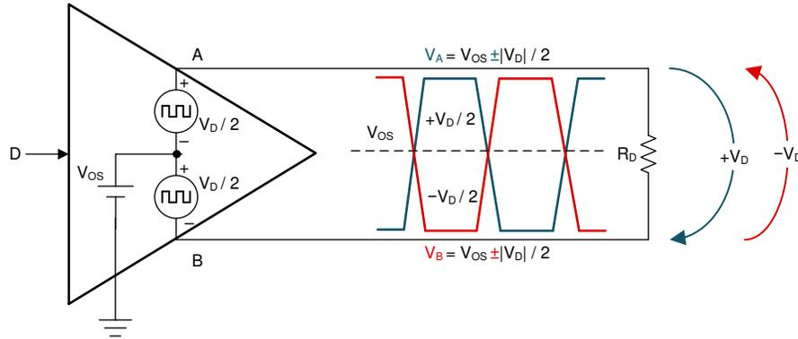
Figure 2-3. RS-485 Driver Output Waveform
