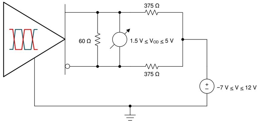
**Figure 3-3. RS-485 Driver-Output Test Circuit With Common-Mode Load**
