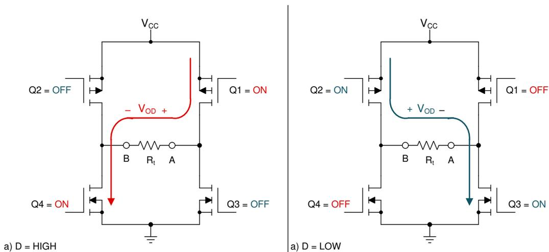
Figure 2-2. RS-485 Output Driver Operation
