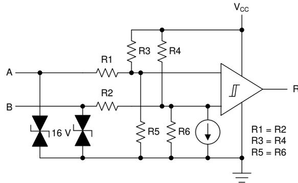
**Figure 4-1. Differential Receiver Input Structure**
