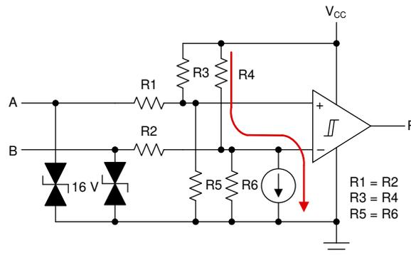
**Figure 4-4. Effect of the Offset Bias Current**
