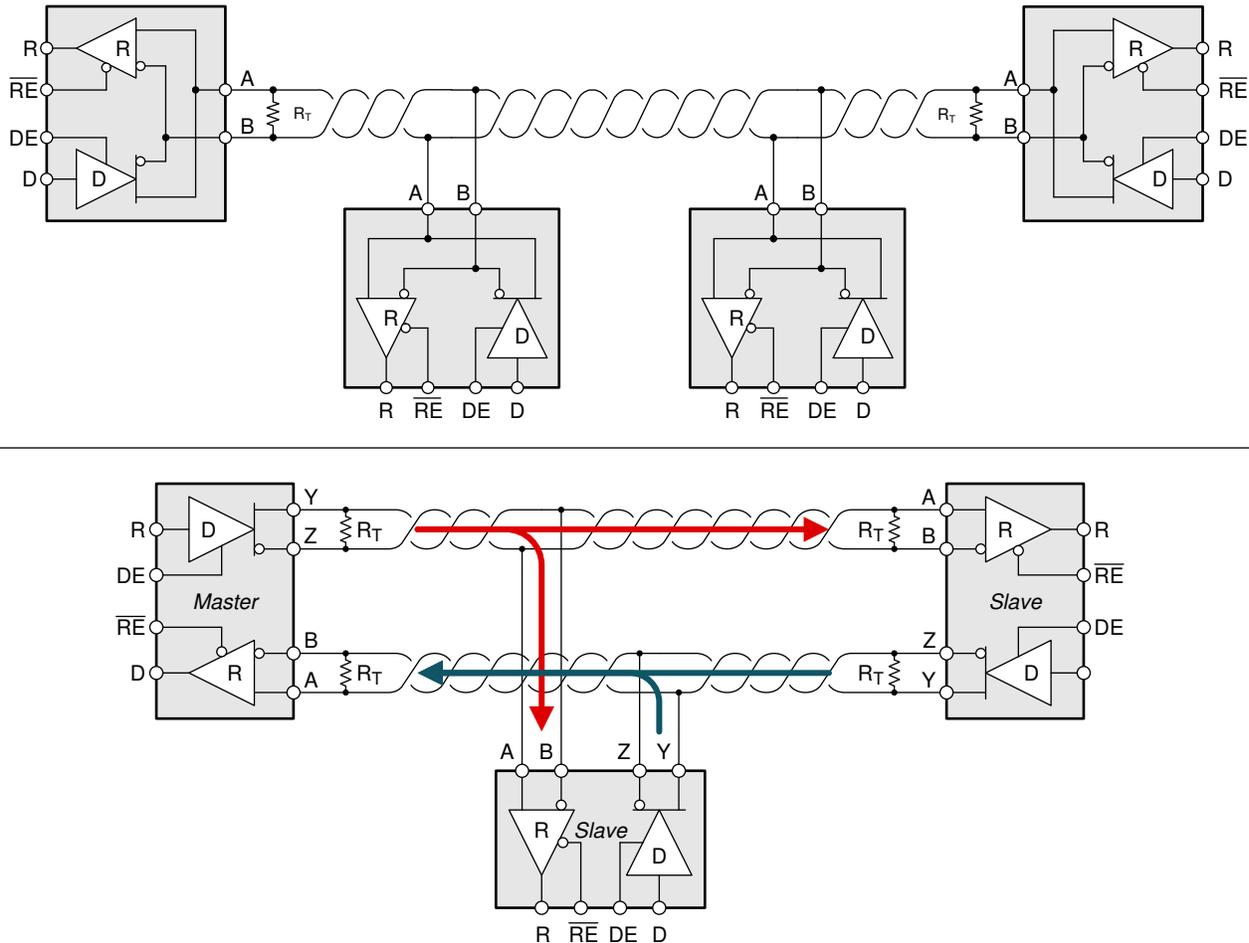
Figure 1-2. Half- and Full-Duplex RS-485 Network Connections
