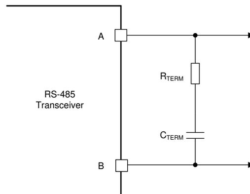
**Figure 6-3. AC Termination Network**
