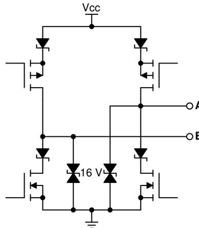
Figure 2-1. Differential Output Driver Structure
