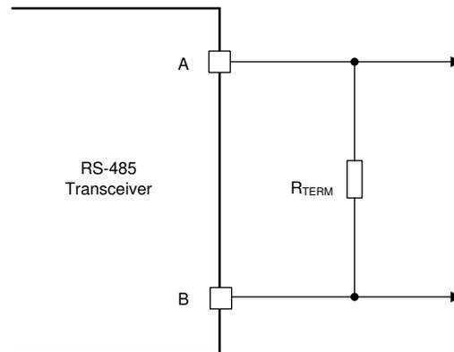
**Figure 6-2. Standard Termination Network**
