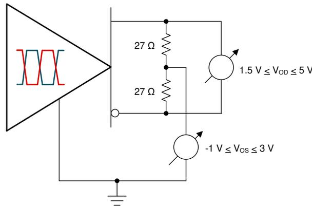
Figure 2-4. RS-485 Output Driver Test Circuit
