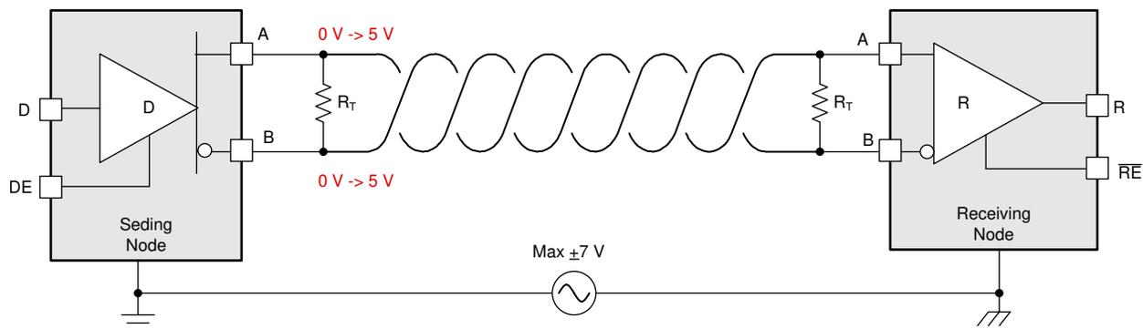
Figure 3-2. Maximum GPD of a Standard RS-485 Transceiver
