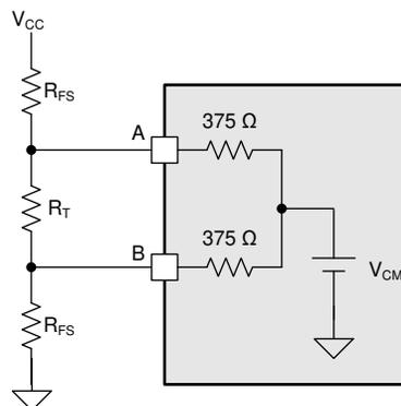
**Figure 5-3. Thirty-Two Unit Loads in Parallel Presenting a Common-Mode Load**
