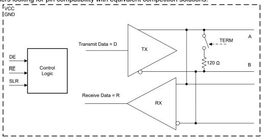
Figure 5-2. THVD1454 Block Diagram
