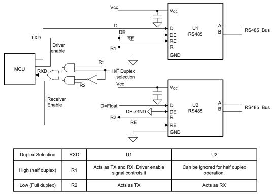
Figure 4-1. Logic Implementation of Duplex Switching
