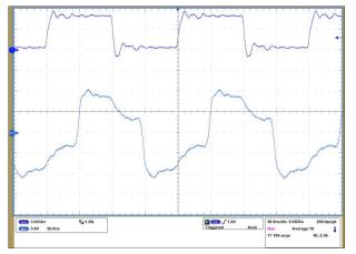
Figure 7-4. Node A and Node D Un-terminated with Signaling at 10 Mbps
