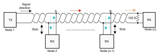
Figure 1-3. Signal Reflection Phenomena in an RS-485 Network
