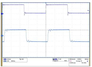
Figure 7-3. Node A and Node D Terminated with Signaling at 2 Mbps
