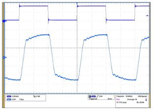
Figure 7-8. Node A and Node D Un-terminated with Signaling at 500 kbps
