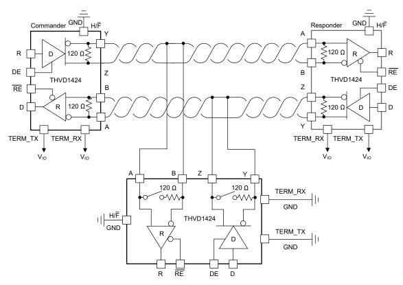
Figure 6-2. Full-duplex Network Using THVD1424
