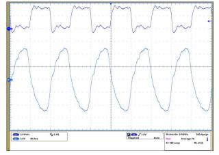
Figure 7-6. Node A and Node D Un-terminated with Signaling at 20 Mbps
