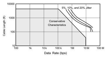
Figure 2-1. Cable Length vs Data Rate Characteristics
