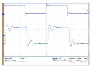
Figure 7-2. Node A and Node D Un-terminated with Signaling at 2 Mbps
