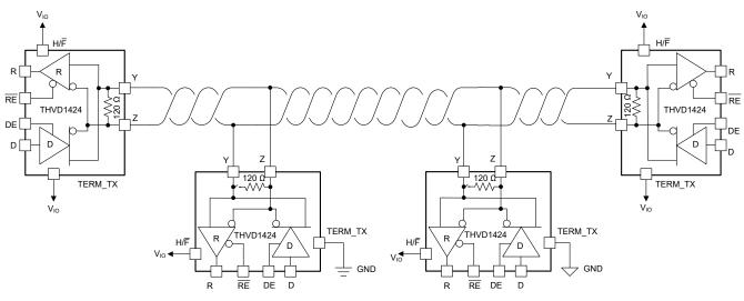
Figure 6-1. Half-duplex Network Using THVD1424
