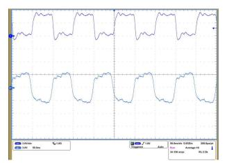
Figure 7-7. Node A and Node D Terminated with Signaling at 20 Mbps
