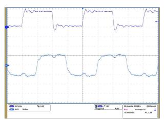
Figure 7-5. Node A and Node D Terminated with Signaling at 10 Mbps
