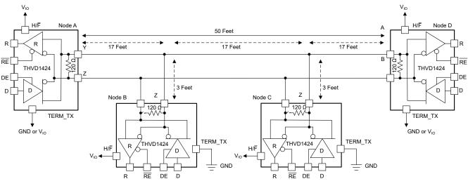
Figure 7-1. Network Set-up with THVD1424
