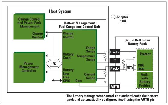
Figure 7. Possible future battery-management architecture enabled by host-side fuel gauging
