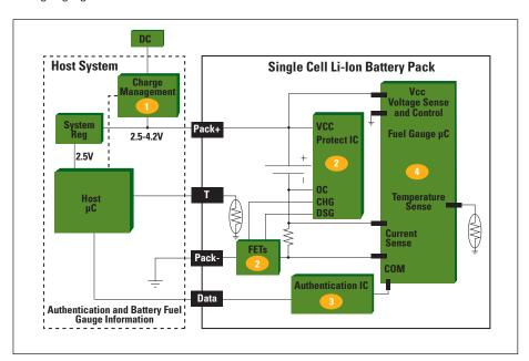
*Figure 1.* The four basic functions of battery management: 1. Charge control, 2. Li-lon protection, 3. Battery pack authentication and 4. Battery fuel gauging
