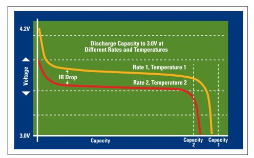
Figure 4a. Rate and temperature dependency on battery discharge capacity
