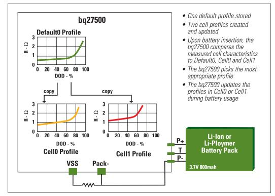
Figure 6. bq27500 "arbitration" method for an inserted battery pack
