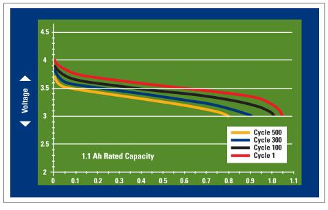
*Figure 4b.* The effect of battery aging (increase in impedance) because of usage on battery discharge capacity
