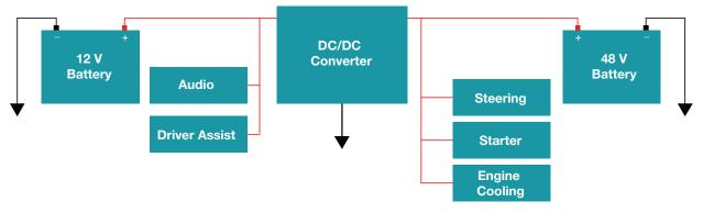
Figure 1. How a 48 V electrical system supports the traditional 12 V system.
