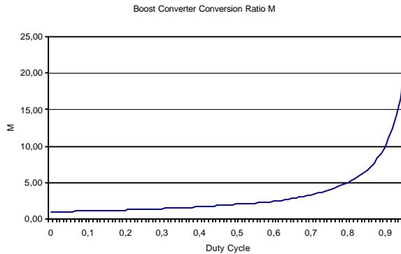
**Figure 3: Variable conversion gains  $M$  of the boost converter**
