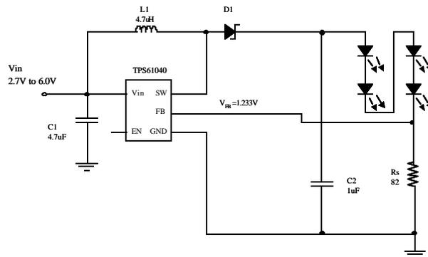
**Figure 4: Boost converter configured as current source**
