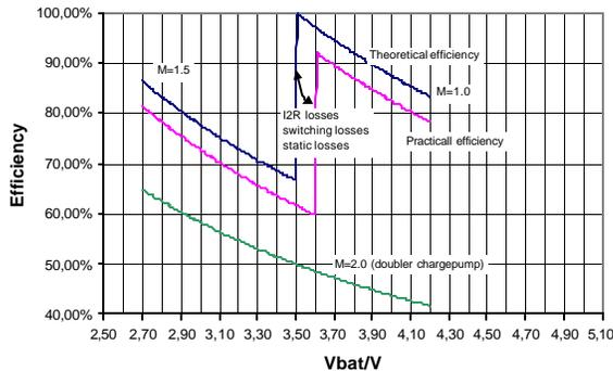
**Figure 2: Efficiency variation of a charge pump solutions**
