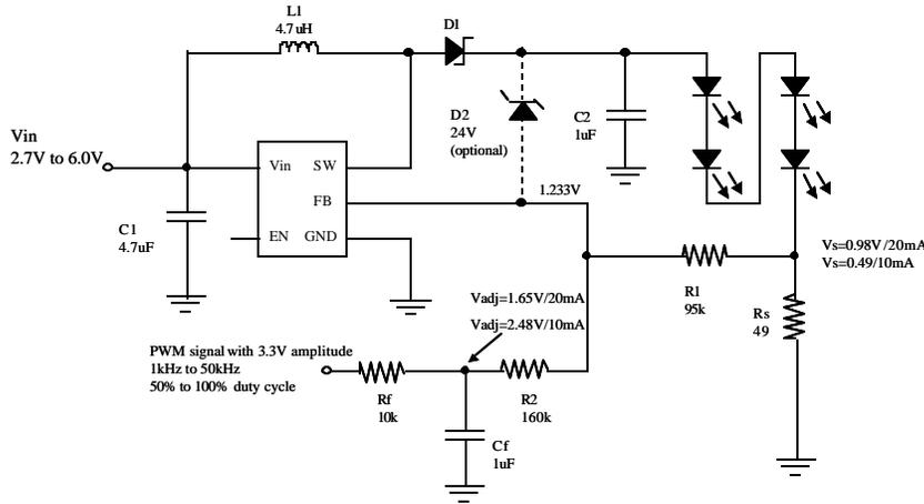
**Figure 5: Increasing the efficiency by lowering the current sense voltage**
