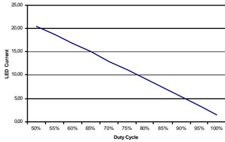
**Figure 7: Simple LED current control by applying PWM signal**
