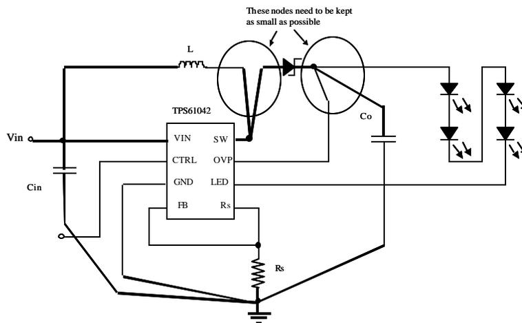
**Figure 11: Nodes and traces carrying switching currents should be kept small**
