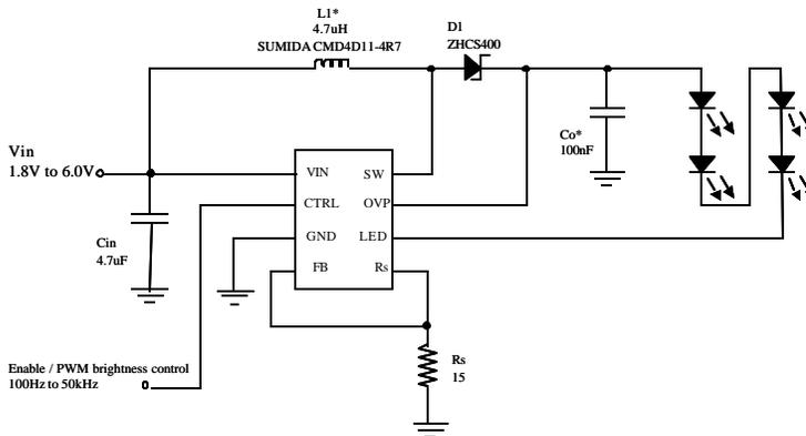
**Figure 8: White LED constant current driver IC**
