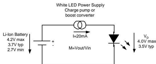
Figure 1: A good efficiency requires a variable conversion gain M
