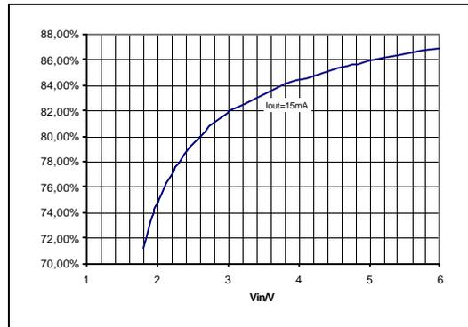
**Figure 10: High efficiency over battery input voltage range**
