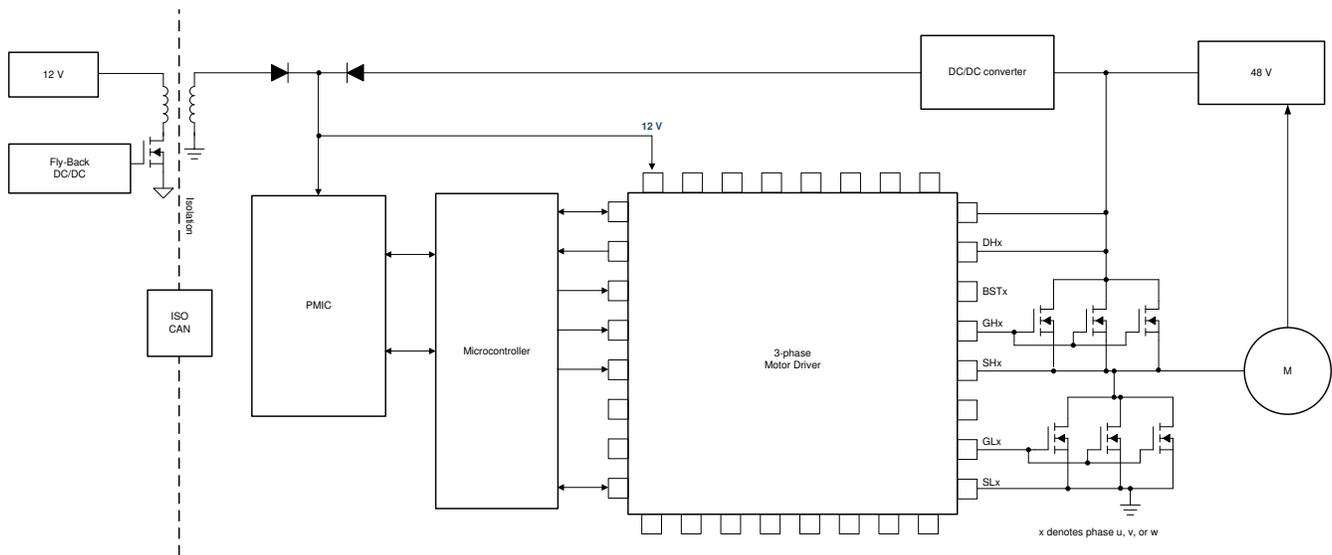
**Figure 3-1. Common Power-Supply Architecture for High-Power 48-V Motor Drivers**
