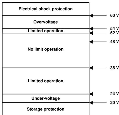
**Figure 3-2. ISO 21780 Specifications for 48-V Voltage Levels**
