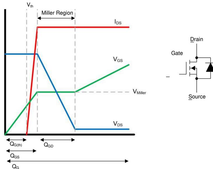
Figure 4-1. Fall Time of  $V_{DS}$  vs Gate Charge
