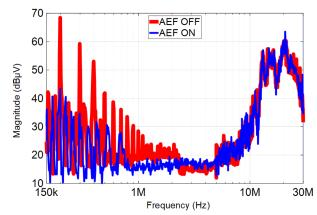
Figure 9-4. EMI Performance With TIDM-1007: AEF Disabled vs. Enabled Using the Same Filter
