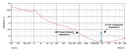
Figure 7-1. Example of Inject Branch Impedance Z<sub>INJ</sub> With AEF Enabled vs. a Conventional Y-Capacitor, Showing the Boosted Equivalent Capacitance at Higher Frequencies by Active Feedback Action
