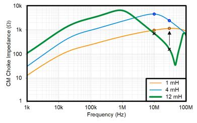
Figure 9-8. Impedance Characteristics of the Selected CM Chokes in the Passive Design (2 × 12 mH) and Active Design (4 mH and 1 mH)
