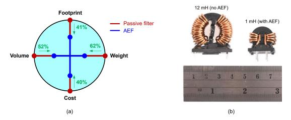
Figure 9-7. Area, Volume, Cost and Weight Reduction Enabled by AEF (a); Choke Size Comparison (b)
