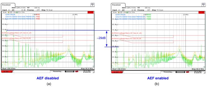
Figure 9-3. EN 55032 Class B EMI Results With AEF Disabled and Enabled
