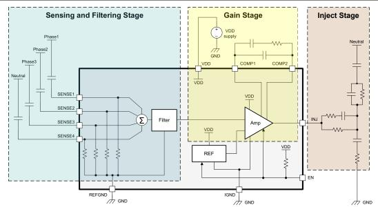
Figure 8-2. Internal Block Diagram of the TPSF12C3-Q1 Three-Phase Stand-Alone AEF IC
