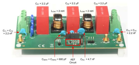
Figure 9-2. Single-Phase Filter Implementation With AEF
