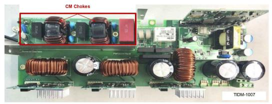
Figure 3-2. Conventional Single-Phase Passive EMI Filter in a Totem-Pole PFC Reference Design
