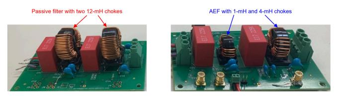
(a) (b) Figure 9-6. Size Reduction Enabled by AEF: Passive Filter (a); Active Filter (b)
