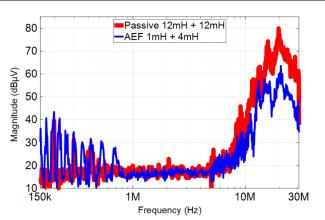
Figure 9-5. EMI Performance with TIDM-1007: A Small-Choke AEF Design Compared to a Large-Choke Passive Filter
