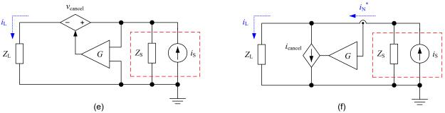
Figure 5-1. Basic Active Filter Structures in Their Single-Phase Equivalents – Four FB and Two FF Circuits – Categorized According to their Control, Sensing and Injection Techniques: FB-CSVI (a); FB-CSCI (b); FB-VSVI (c); FB-VSCI (d); FF-VSVI (e); and FF-CSCI (f)
