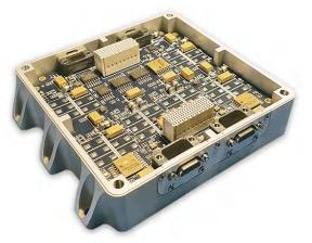
Figure 1-3. STAR-Tiger Power-Supply Board
