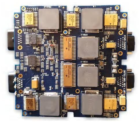
Figure 2-2. STAR-Tiger Power-Supply Board
