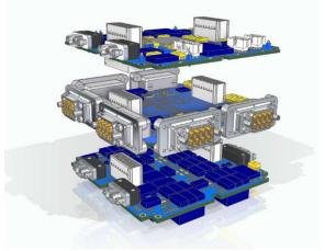
Figure 1-2. STAR-Tiger Routing Switch Board Arrangement
