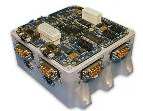
Figure 1-5. STAR-Tiger Configuration Board in Housing
