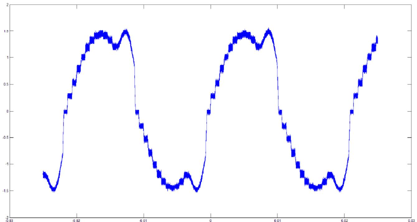
**Figure 5. Shows loss of current regulation in the presence of BEMF**
