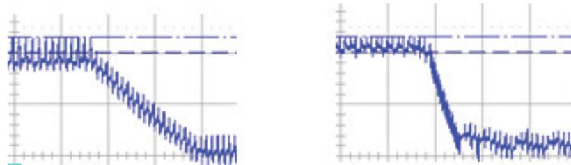
**Figure 7. A 600 uS step transition in fixed decay vs 200 uS transition in smart tune adaptive decay mode**
