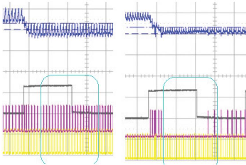
**Figure 8. Fixed mixed decay versus smart tune**
