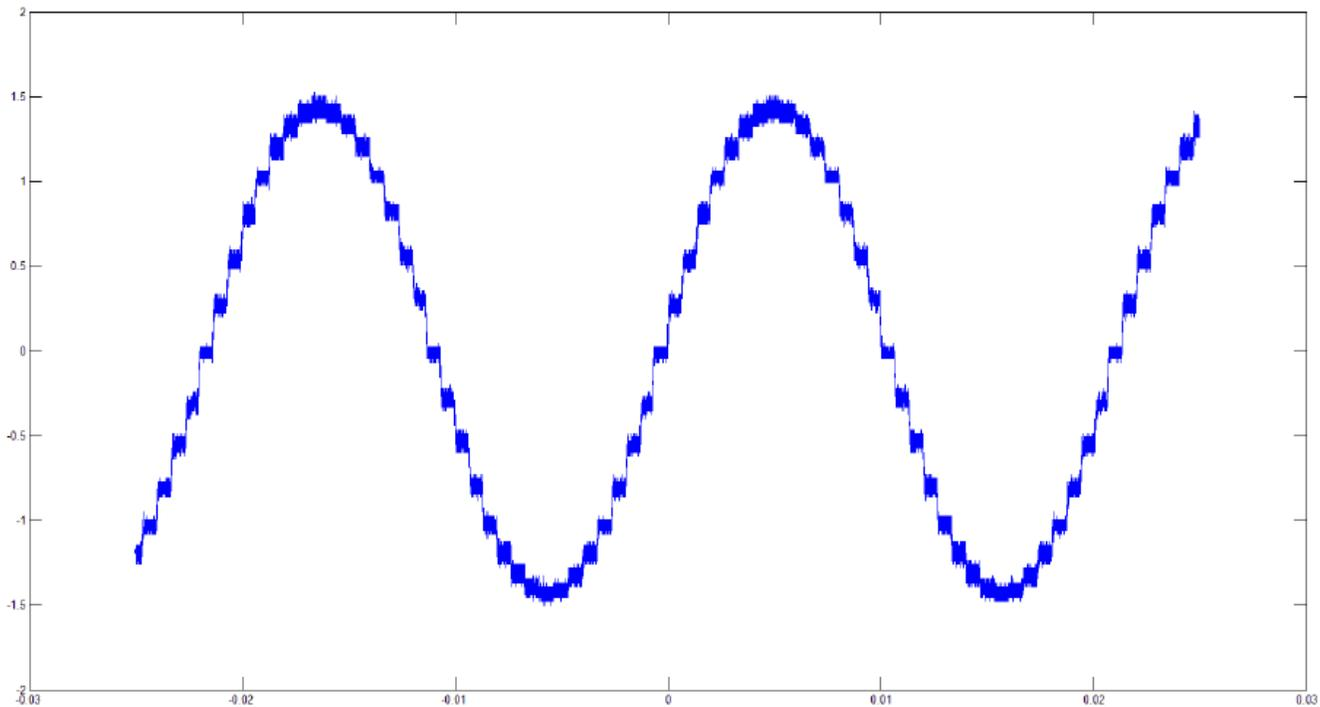
**Figure 6. This chart shows how a stepper motor with adaptive decay tames BEMF**
