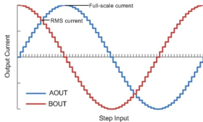
Figure 1. Sine and cosine functions of micro-stepping
