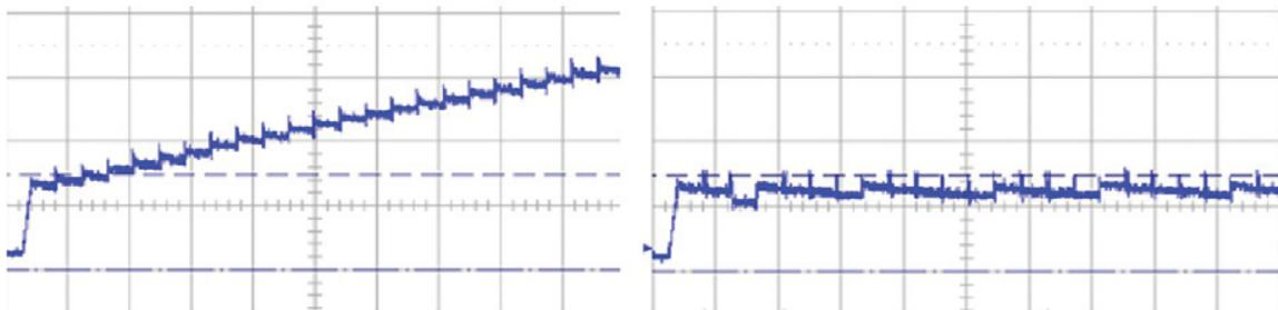
**Figure 9. Fixed slow decay mode versus smart tune on TI's DRV8846**
