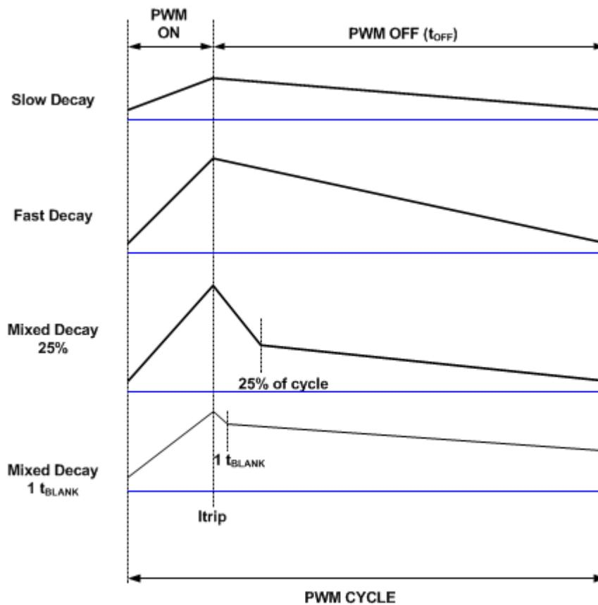
**Figure 3. Current waveforms in slow, fast and mixed decay modes**
