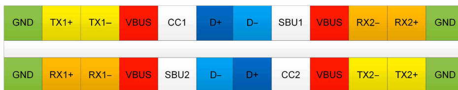
Figure 13. Type-C receptacle pinout.
