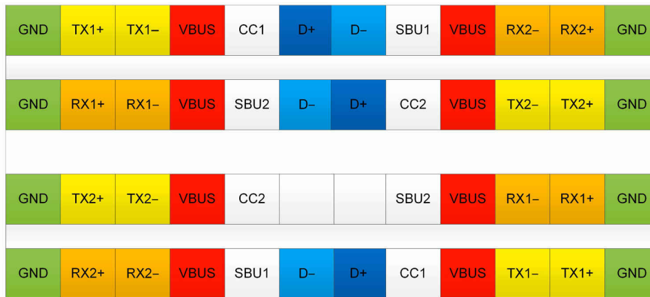
Figure 14. Type-C pinout – receptacle (top), plug (bottom).
