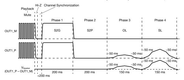
Figure 6. Load-diagnostic output waveforms timing diagram
