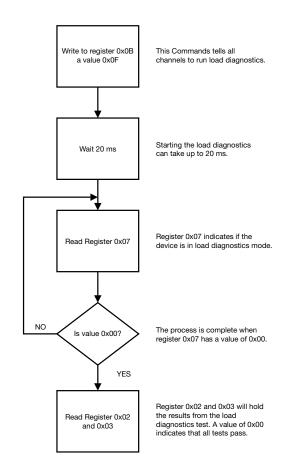
Figure 5. Load diagnostics for four channel amplifiers
