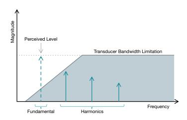
Figure 10. Bandwidth limitations of microspeakers and how smart bass can improve perceived bass
