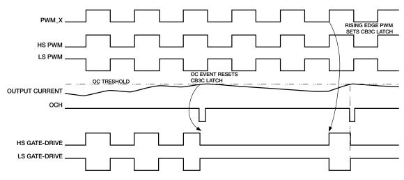
Figure 1. TPA3251 OCP timing diagram
