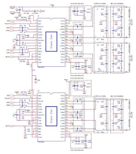
Figure 4. Typical 2.1 channel master/slave application with SYNC pin enabled
