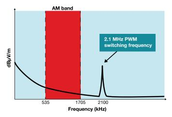
Figure 2. 2.1 MHz PWM switching frequency
