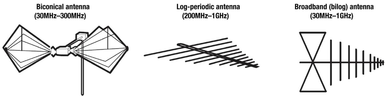
**Figure 3.** Measurement antennas referenced in the CISPR 25 specification.
