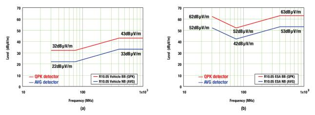
Figure 1. UNECE Regulation 10 radiated EMI limits for vehicles at 10m (a); and ESAs/components at 1m (b).
