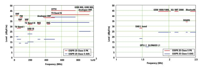
*Figure 2.* CISPR 25 Class 5 radiated limits for components/modules using the Absorber-Lined Shielded Enclosure (ALSE) test method with an antenna distance of 1m.
