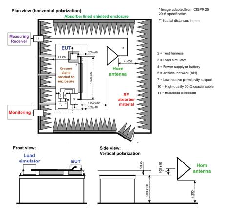
Figure 6. CISPR 25 radiated emissions measurement setup with horn antenna (above 1GHz).
