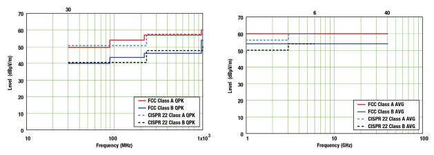
*Figure 7.* FCC Part 15 and CISPR 22/32 radiated limits for Class A and Class B using QPK and AVG detectors below and above 1GHz, respectively.
