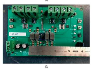
Figure 6. Power-density comparison at 120 A: four competitor modules current sharing (a); one TPSM831D31 module (b).
