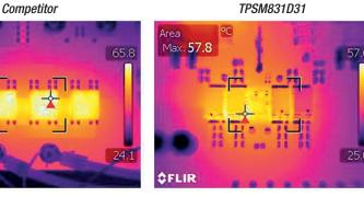
Figure 3. Thermal performance comparison:  $V_{IN} = 12 V$ ,  $V_{OUT} = 1.0 V$ ,  $I_{OUT} = 100 A$ ,  $F_{sw} = 500 kHz$ , 22°C ambient, 200 linear ft./min. airflow.
