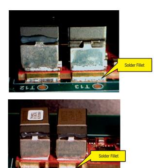
Figure 15. TPSM831D31 module edge plating.
