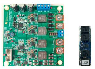
*Figure 14.* Discrete regulator vs. the TPSM831D31 (four total phases in each design).
