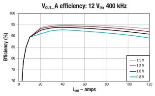
Figure 9. TPSM831D31 module channel at 120-A efficiency.
