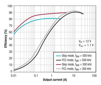
*Figure 7.* TPS53119 efficiency plot; skip and forced continuous conduction (FCC) mode operation.
