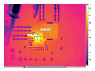
Figure 5. TPS548B22 thermal performance,  $T_{max} = 66.3$ °C.
