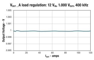
Figure 11. TPSM831D31 DC load regulation up to 120 A.
