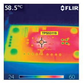
Figure 4. TPS53119 thermal performance,  $T_{max} = 58.5$  °C.
