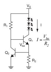
Figure 8. A current-source LED circuit with two transistors.
