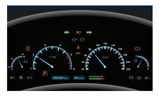
Figure 1. Instrument cluster dashboard indicators.
