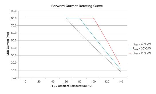
Figure 3. Example LED current derating curve.
