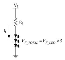
Figure 4. Direct LED drive with R<sub>s</sub>.
