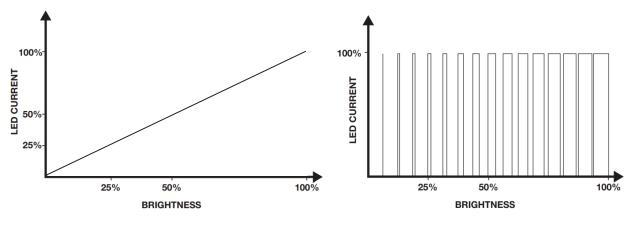
Figure 11. Analog dimming vs. PWM dimming.
