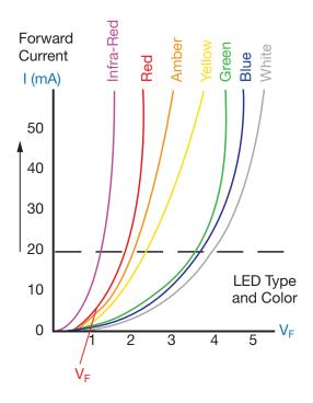
Figure 2. LED V<sub>E</sub> vs. I<sub>E</sub>.
