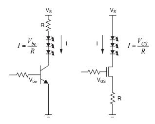
Figure 5. Constant-current LED drive with transistors.
