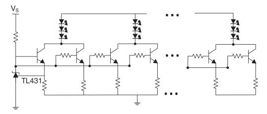
Figure 9. Driving multiple LED strings with discrete components.
