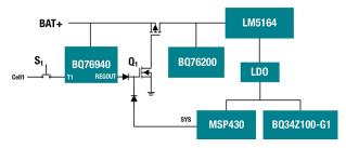
Figure 2. Auxiliary power-supply block diagram.
