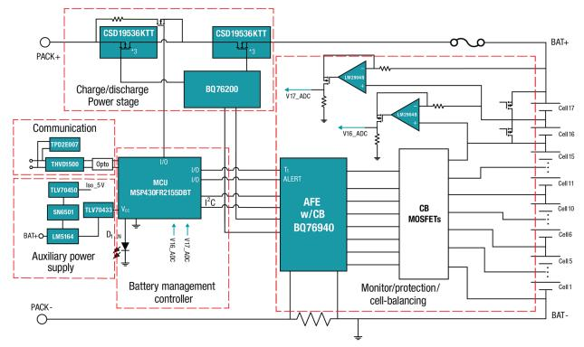
Figure 3. The 16S-17S battery pack reference design.
