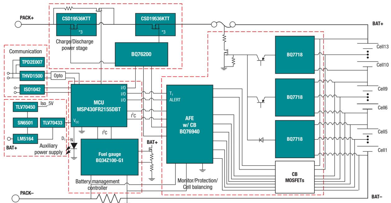
Figure 1. The accurate gauging reference design.
