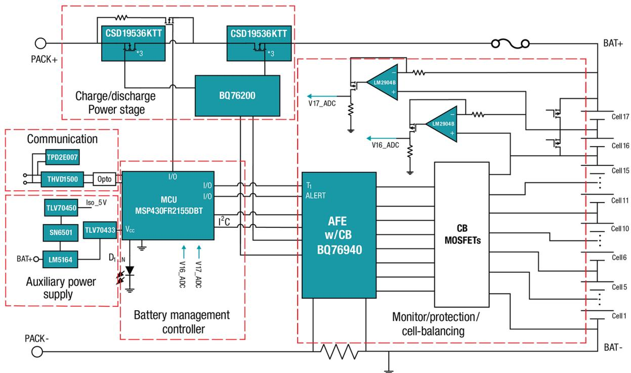
**Figure 3.** The 16S-17S battery pack reference design.
