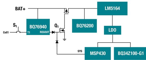
**Figure 2.** Auxiliary power-supply block diagram.
