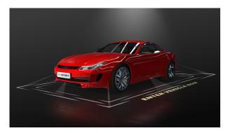
*Figure 3.* Automotive light carpet projected from multiple locations on the vehicle.
