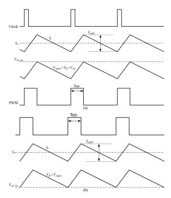
**Figure 10.** AECM control scheme waveform: PWM operation mode (a); PFM operation mode (b).
