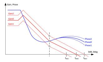
**Figure 6.** Bode plot with different VOUT conditions of a D-CAP2 $^{\text{TM}}$  buck converter.
