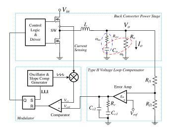
Figure 1. PCM control scheme block diagram.
