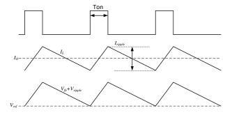
Figure 4. D-CAP2 control scheme waveform.
