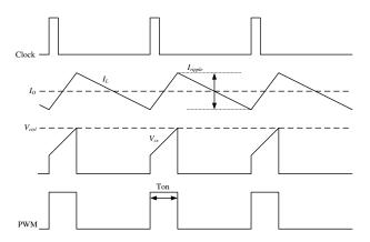
Figure 2. PCM control scheme waveform.
