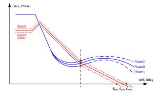
**Figure 13.** Bode plot under different  $V_{OUT}$  conditions of AECM.
