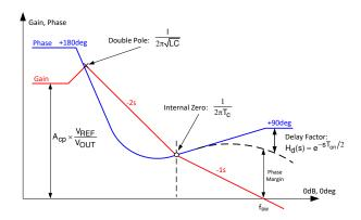
Figure 5. Bode plot with different VOUT conditions of a D-CAP2 buck converter.
