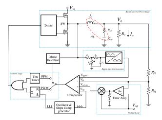
Figure 9. AECM control block diagram.
