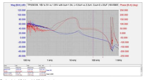
Figure 14. Measured Bode plot of 5-V and 1.05-V outputs.
