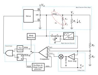
Figure 7. AECM control block diagram.
