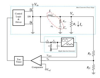
Figure 3. D-CAP2™ control scheme block diagram.
