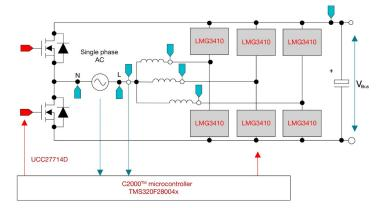
**Figure 3**. The GaN CCM totem pole reference design employs digital control using a C2000 real-time MCU and a fast switching GaN device with integrated gate-driver and protection features.
