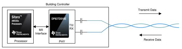
SPE Interface for 10 Mbps Using the DP83TD510E
