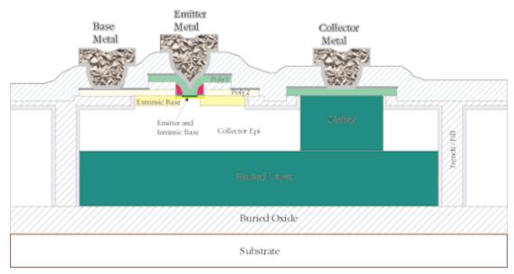
Figure 1: VIP10 Transistor Cross Section
