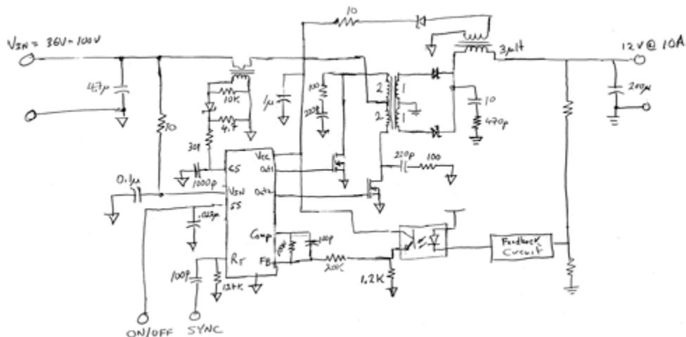
Figure 1: Push-Pull Converter
