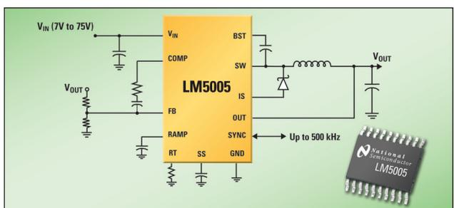
The LM5005 is available in a power enhanced TSSOP-20 package featuring an exposed die attach pad to aid thermal dissipation. It is ideal for use in consumer electronics, telecommunications, data communications systems, automotive power systems, and distributed power applications.
