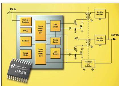
The LM5032 and LM5034 are flexible controllers that can be configured to control either two independently regulated outputs or a single, high-current output from two
