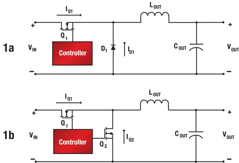
Figure 1. (a) Non-synchronous and (b) synchronous buck converters.
