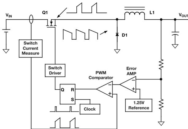
**Figure 1.** Buck regulator using current mode control.
