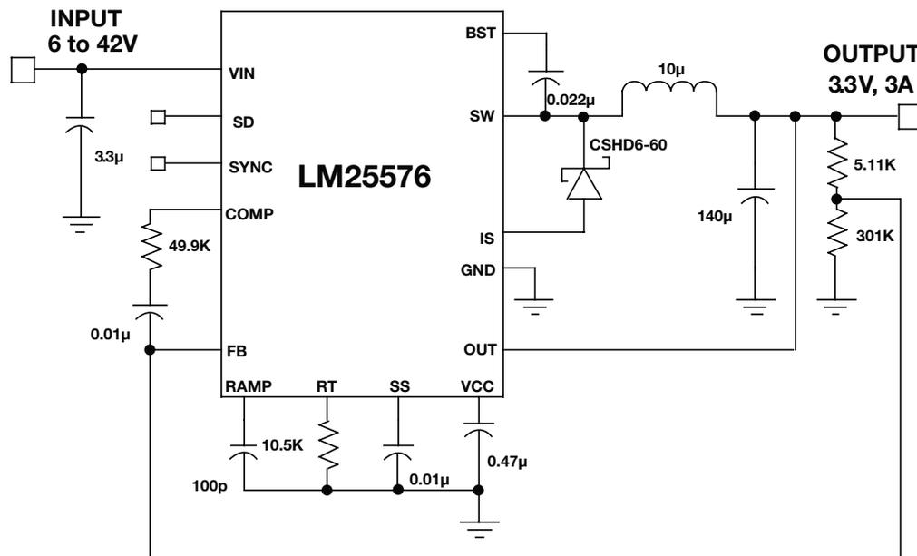
**Figure 4.** LM25576 buck regulator schematic.
