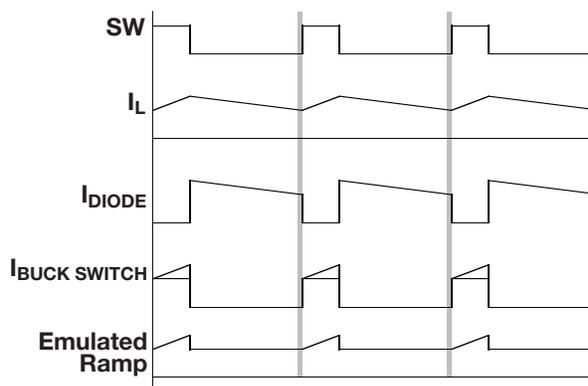
**Figure 2.** Buck regulator waveforms.
