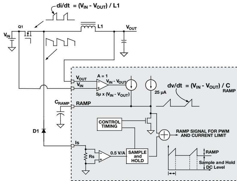
**Figure 3.** Emulated current mode control ramp generator.
