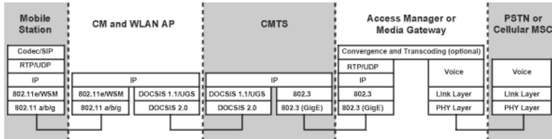
**Figure 3: End-to-end voice bearer protocol stack**
