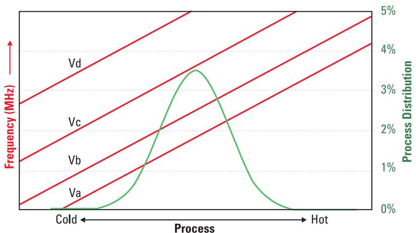
Figure 3. Dependency on voltage.
