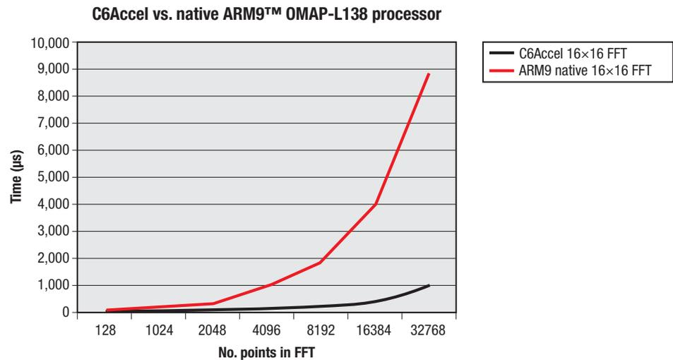
Figure 4. Graph of execution time vs. data size while using C6Accel and ARM for data processing.
