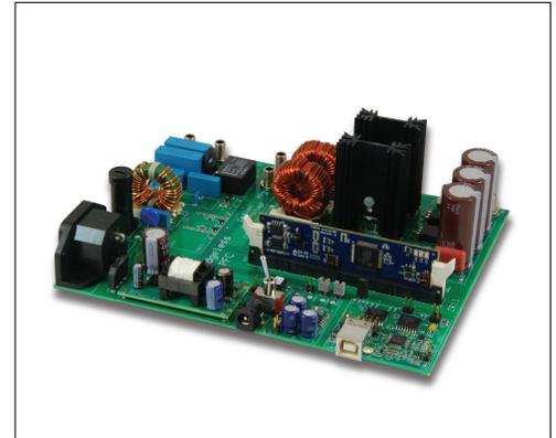
▲ **Fig. 2b** – High Efficiency (Bridgeless) PFC Developers Kit
