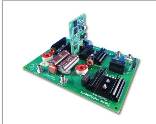
▲ **Fig. 2a** – High Voltage 2-Phase Interleaved PFC
