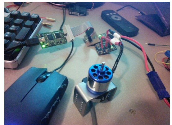
Figure 7. 2278 1000Kv motor with Custom FOC Controller.
