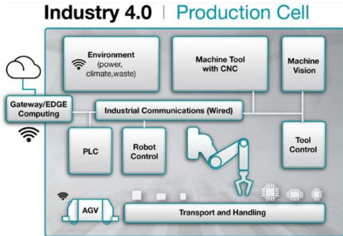
**Figure 1.** Industry 4.0 production cell with TSN backbone.
