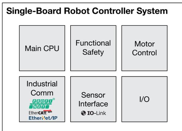
**Figure 5:** Single-board robot controller system for collaborative or SCARA robots.
