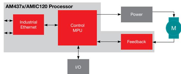
**Figure 6:** Single-chip robot controller system based on AM437x or AMIC120 processors.
