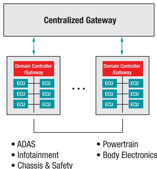
**Figure 1.** Example SoC architecture, featuring a centralized gateway and two domain gateways.
