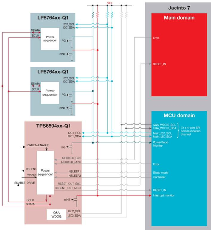
Figure 3. TPS6594-Q1 + LP8764-Q1 + LP8764-Q1 Communication as “Virtual” PMIC
