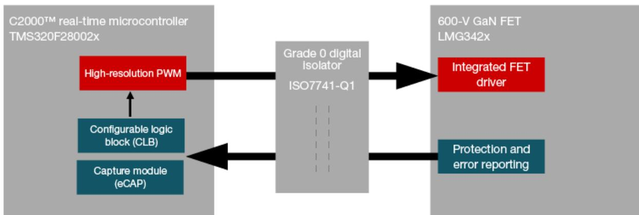
**Figure 4.** The only components needed to interface a C2000 MCU with a TI GaN device.
