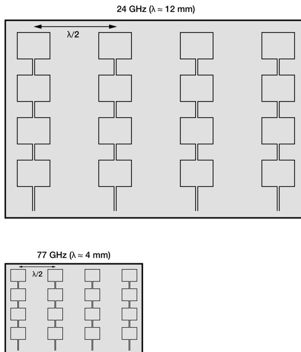
**Figure 3.** The 77-GHz antenna array is significantly smaller than the 24-GHz antenna array.
