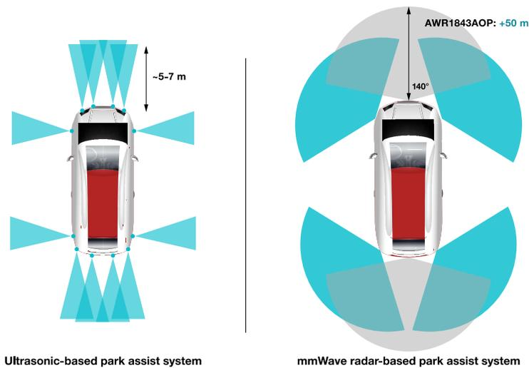
**Figure 5.** Comparison of range and field of view for ultrasonic vs. mmWave radar systems.
