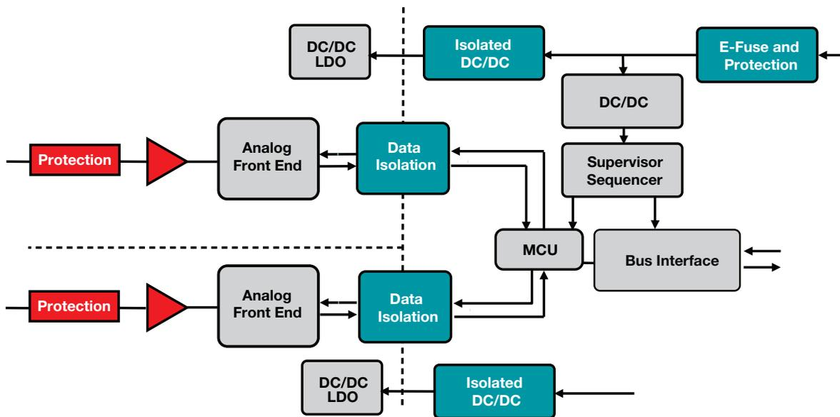
Figure 1. PLC with isolation
