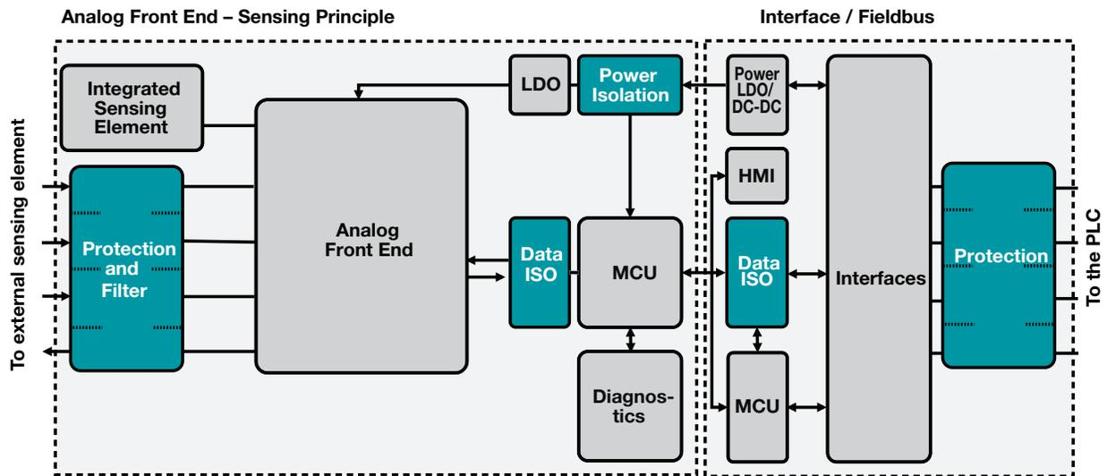
Figure 2. Sensor with isolation
