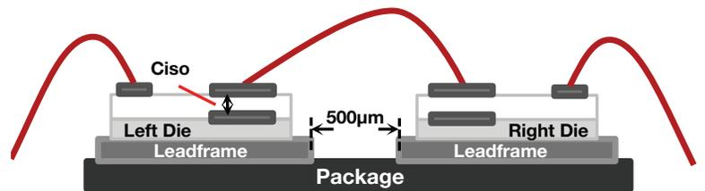
Figure 3. Block diagram of MCM with isolation capacitors
