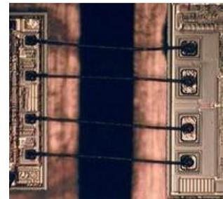
Figure 4. Photo of MCM with isolation capacitors
