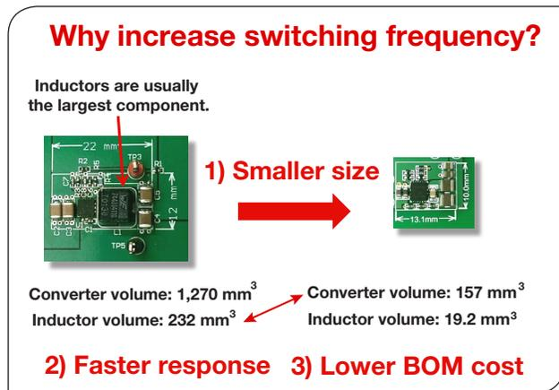
Figure 4. Rescaling buck converter designs
